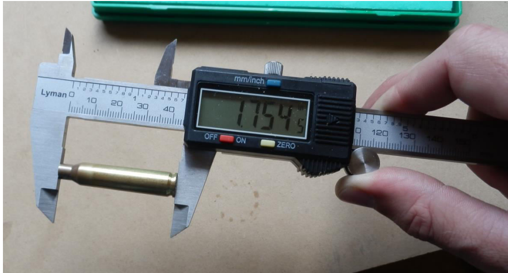
Figure 3.15. Case length measurement with digital caliper.
