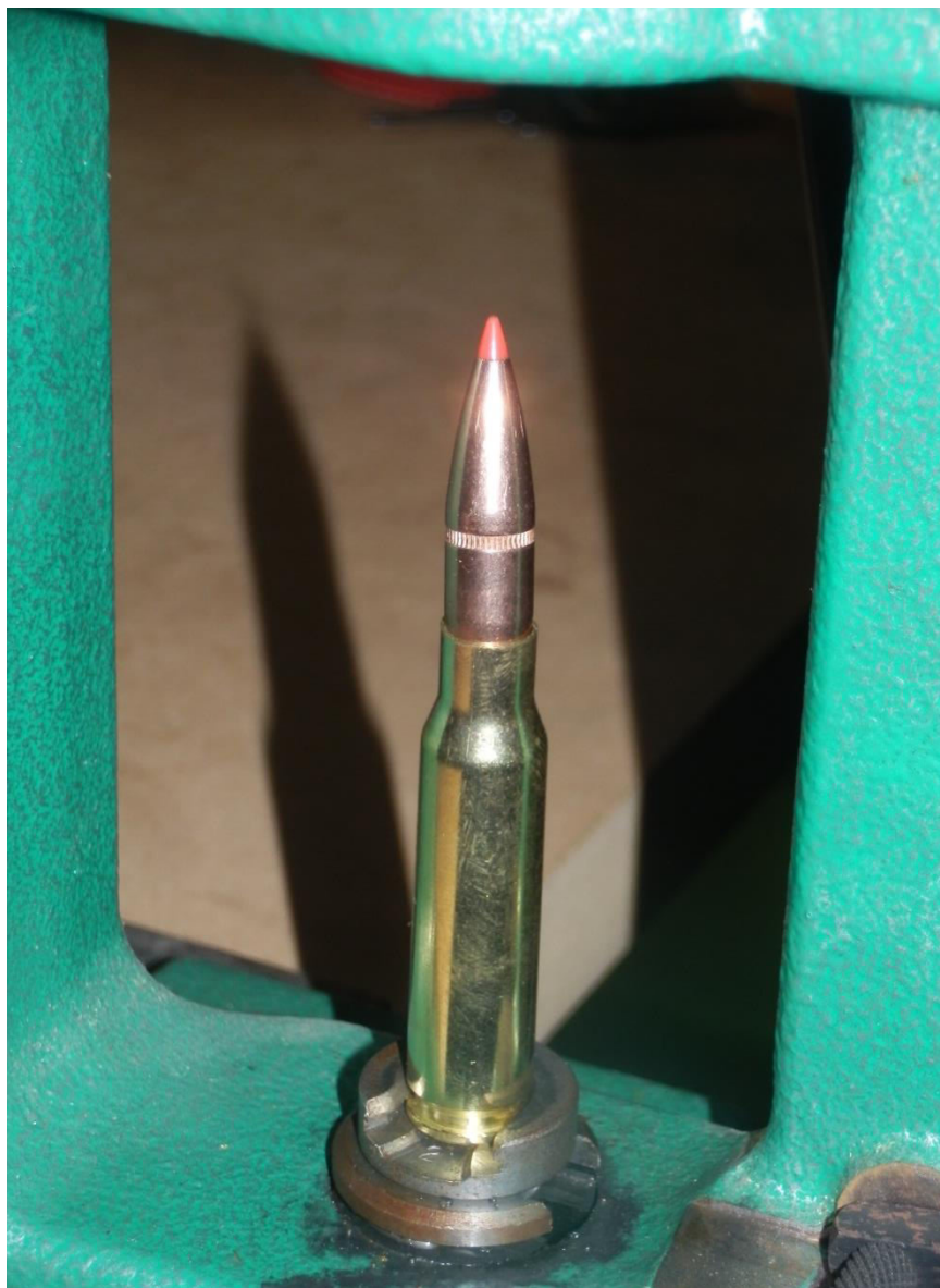
Figure 3.19. .308 Winchester cartridge in reloading press prior to bullet seating.
