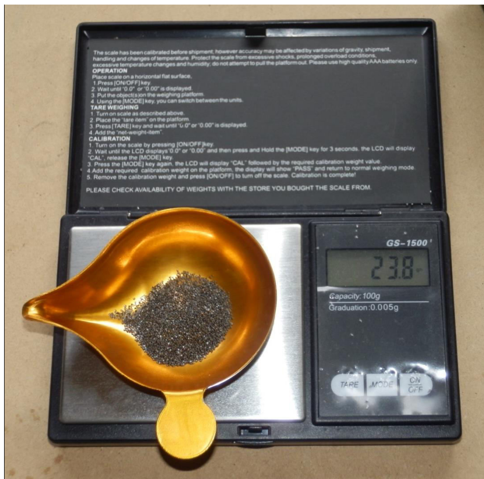
Figure 3.17. Digitally weighing powder load.
