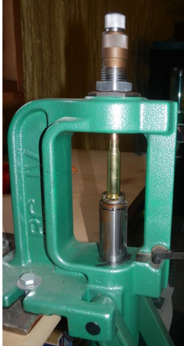
Figure 3.20. .308 Winchester cartridge being pressed in to seating die.
