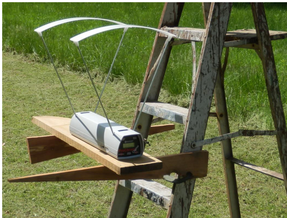
Figure 3.23. ProChrono on ladder stand with diffusers mounted.
