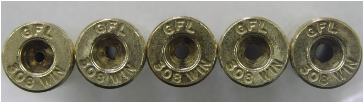
Figure 1.4. Left to right, 1.4mm, 2.0mm, 2.4mm, 2.8mm, 3.0mm flash holes drilled in .308 Winchester cases.
