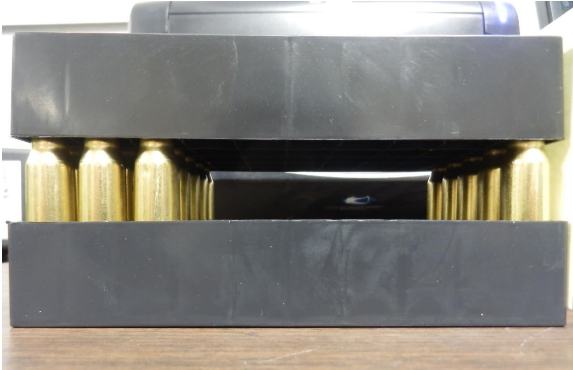
Figure 3.28. .308 cartridges sandwiched in ammo wells so they could be rotated.
