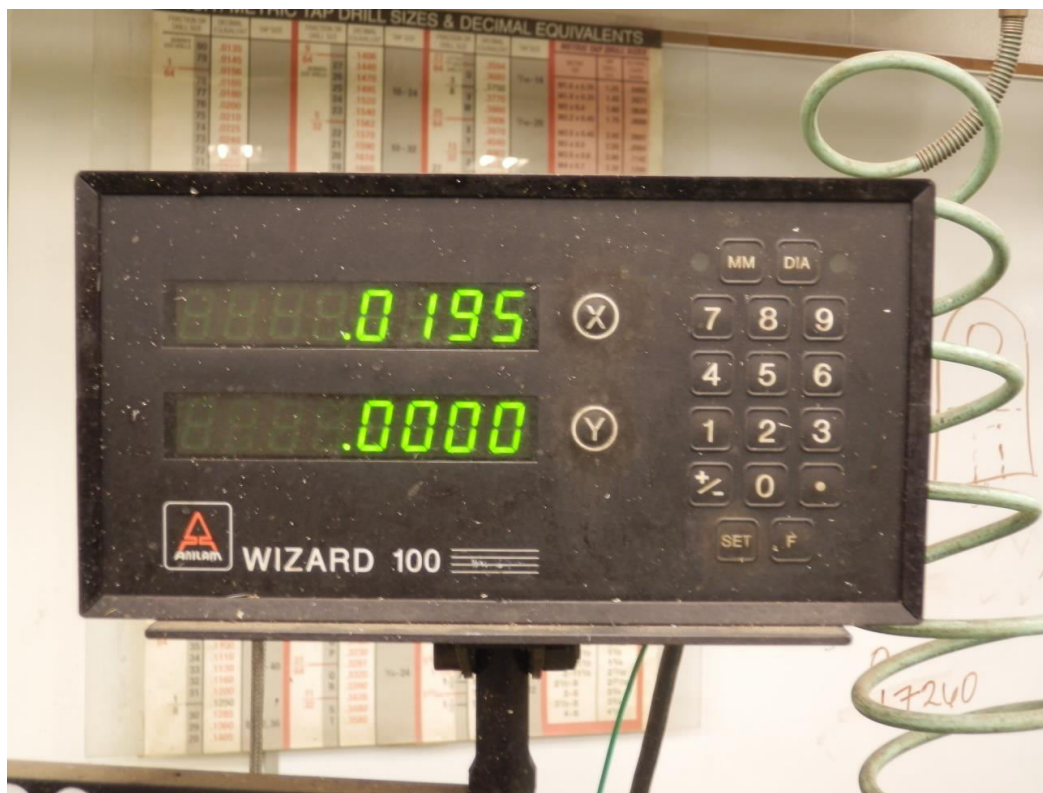
Figure 3.7. Drill offset 0.0195in (0.5mm).
