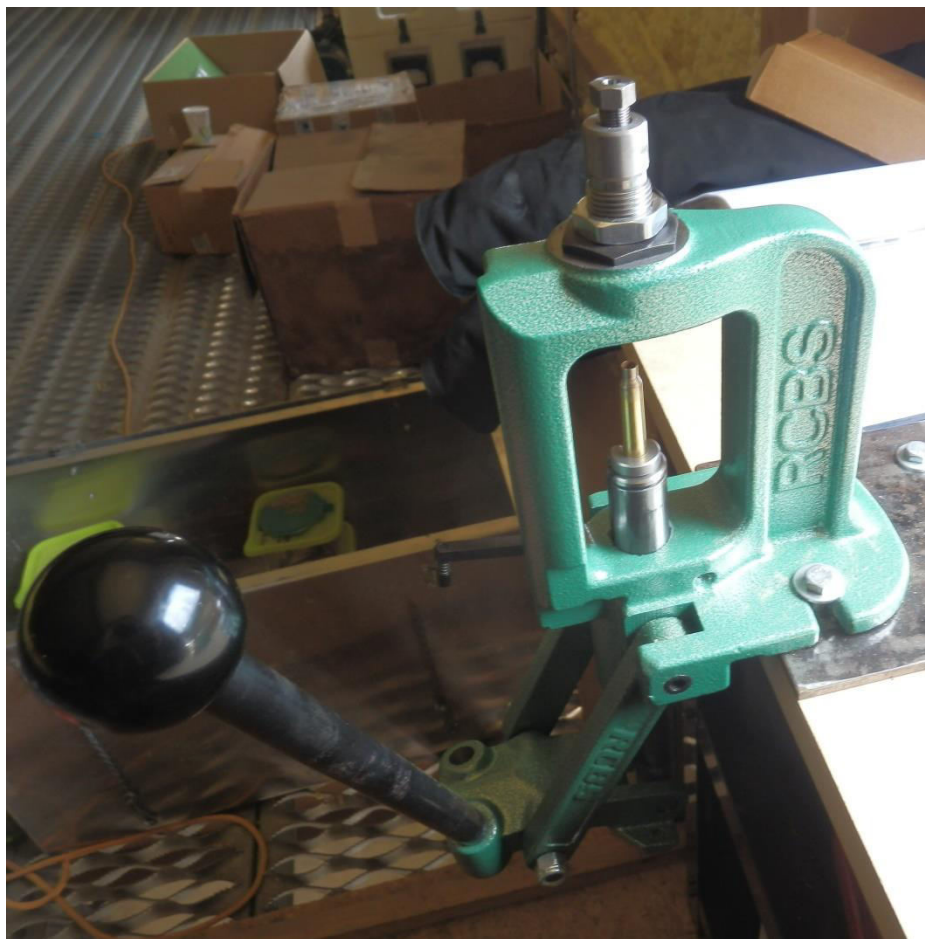
Figure 3.12. Case in press with sizing die.
