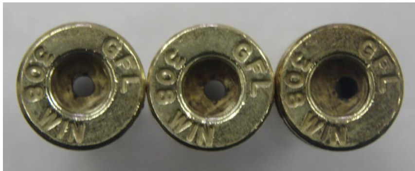
Figure 1.5. Left to right, Centered, offset 0.5mm, offset 1.0mm flash holes with 2mm diameters.
