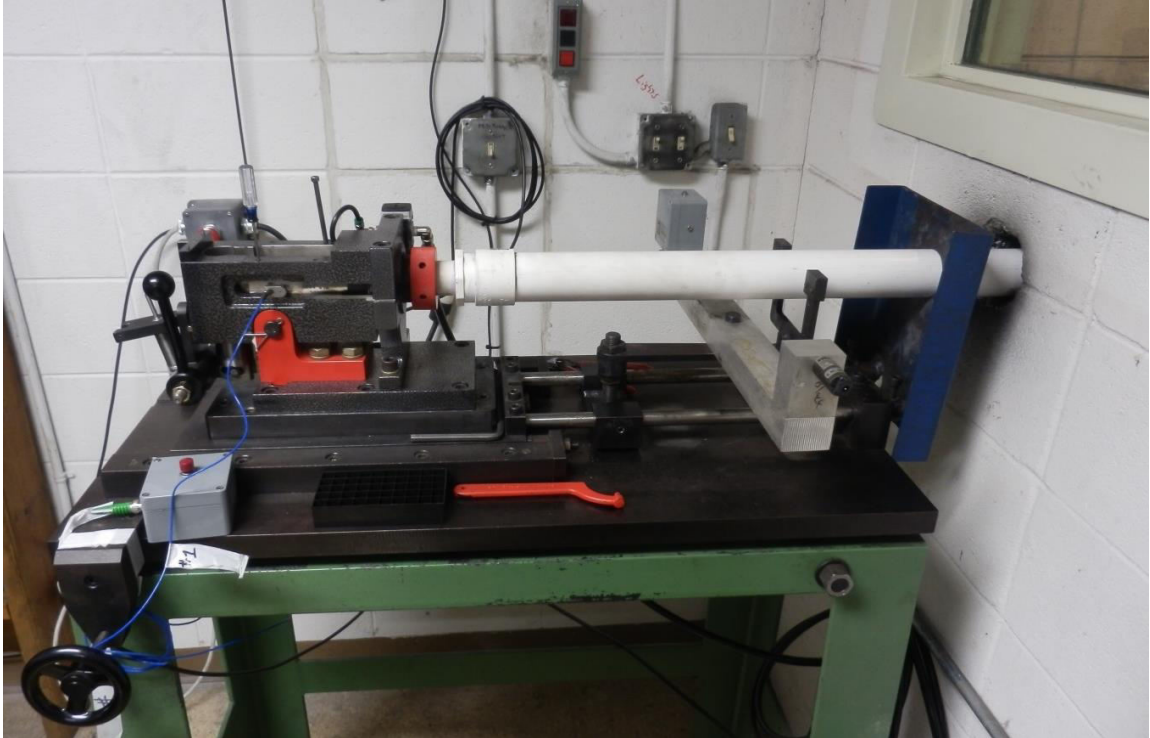
Figure 3.25. Bench rifle setup in recording room at Fiocchi of America.
