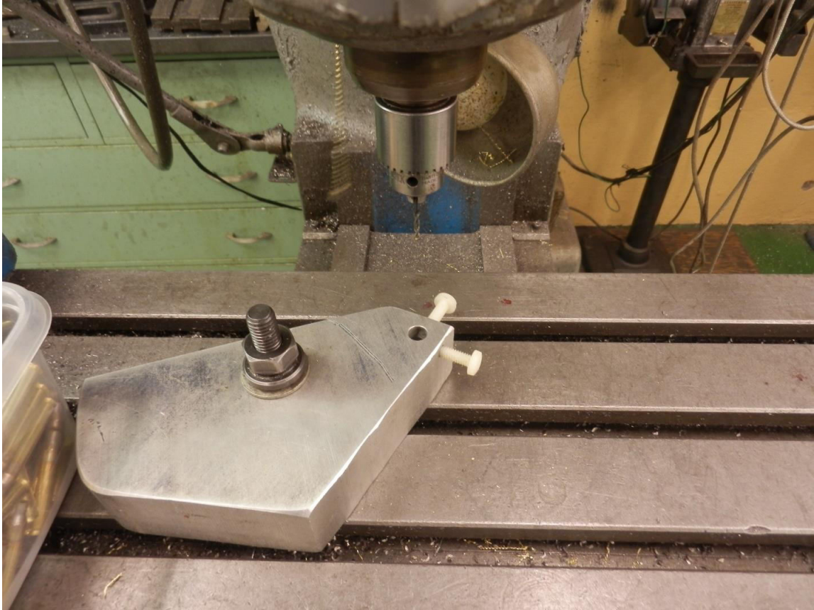
Figure 3.6. Anchored down aluminum block ready for drilling.
