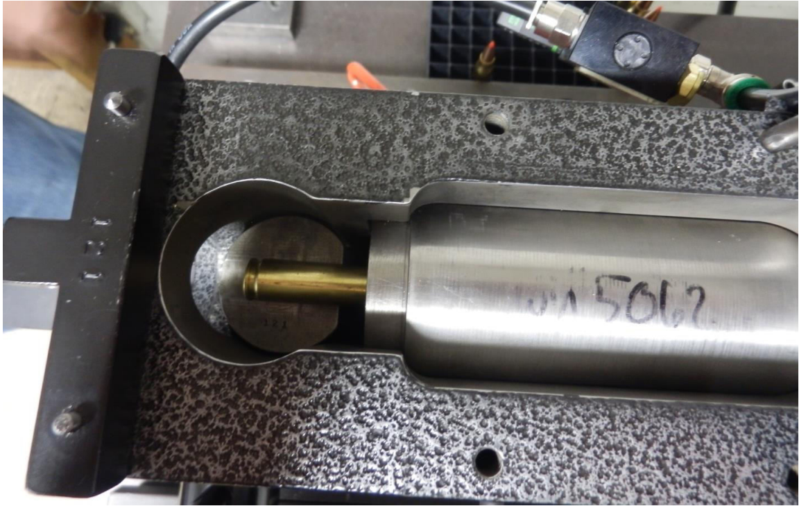
Figure 3.30. .308 cartridge partially loaded into bench rifle chamber, top view.
