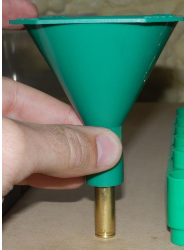
Figure 3.18. Funnel measured powder load into case.
